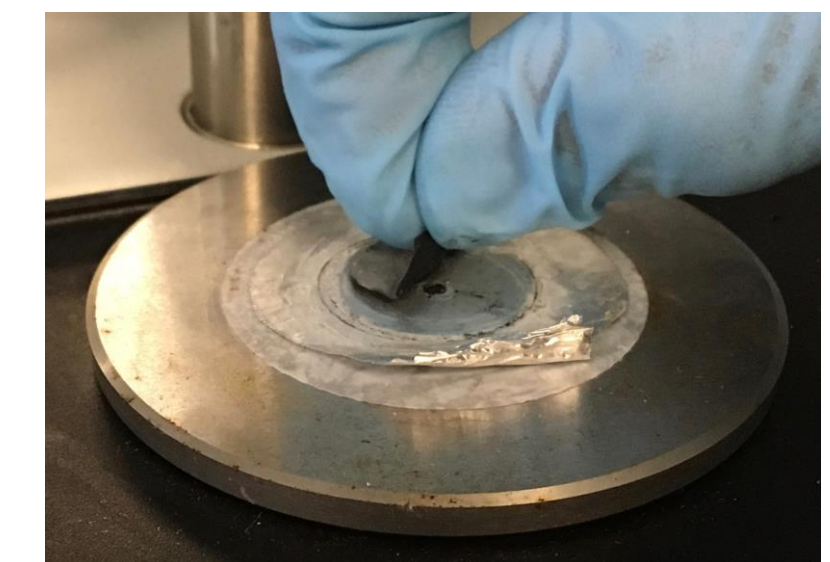
The battery is positioned atop a diamond crystal, which directs infrared light into the battery.
